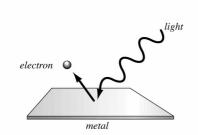
When light is shone at certain materials, a small current is produced as the energy from the photons (packets of energy) is tranferred to electrons - freeing them from their positions.
