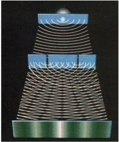
The photosensitive detector shows bands of light reaching it suggesting that the 2 waves interact with their peaks and troughs to produce a detection or cancel it to produce no detection.
