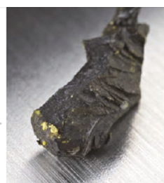
▶ Europium (Eu), is one of the lanthanoids. It is a hard silvery-white metallic element and is used in television screens and fluorescent light bulbs.
