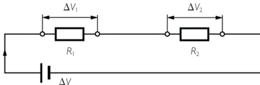
The current going through the first resistor will also go through the second resistor. Therefore, the intensity or current going through all the resistors is the same.
