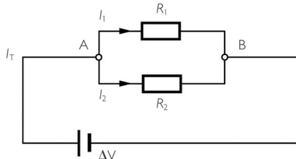
Once the current gets to point A, it splits up and some will flow through the upper branch, going through  $R_1$ , and the rest will flow through the lower branch, where we find  $R_2$ . However, as electric charge is conserved, the total intensity is the sum of all of the individual intensities.
