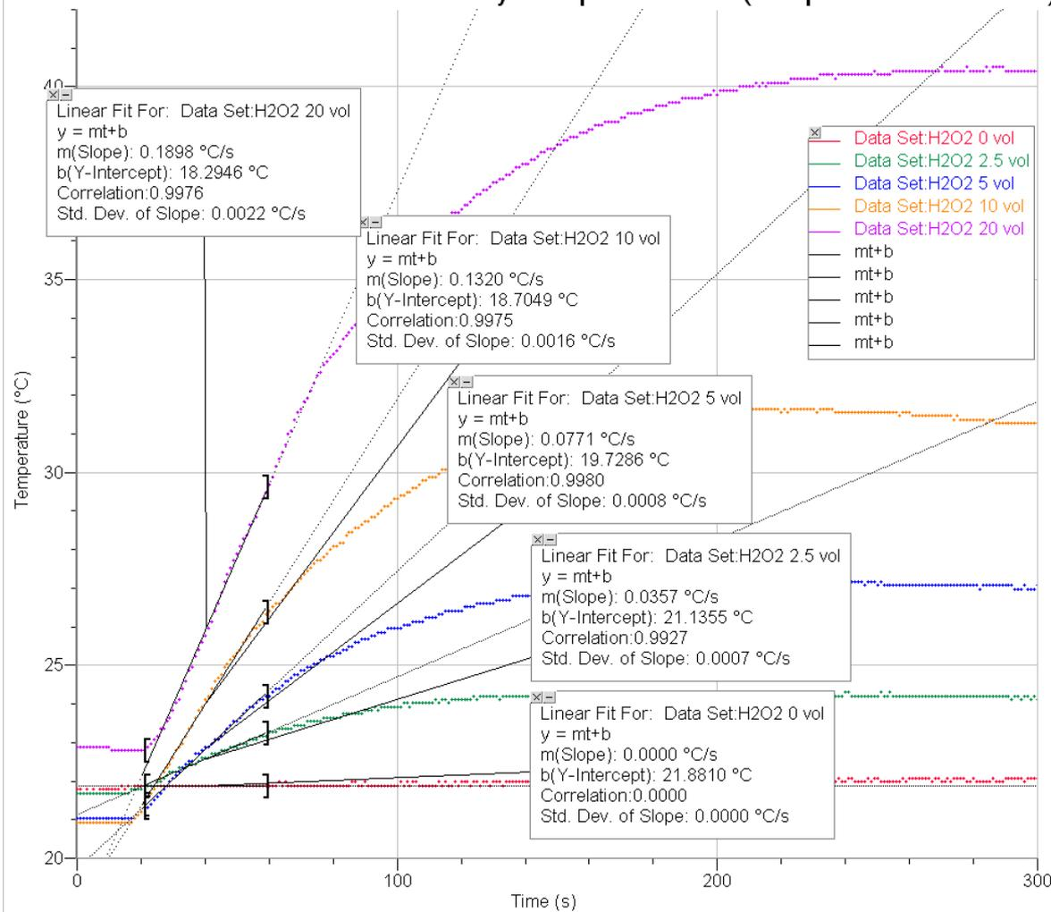
The initial reaction rates obtained are taken from the graph and put into Excel.
