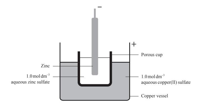
The porous cup allows the movement of ions between the two solutions, while preventing physical mixing. The standard potential of the cell,  $E_{cell}^{\circ}$ , is 1.10 V.
