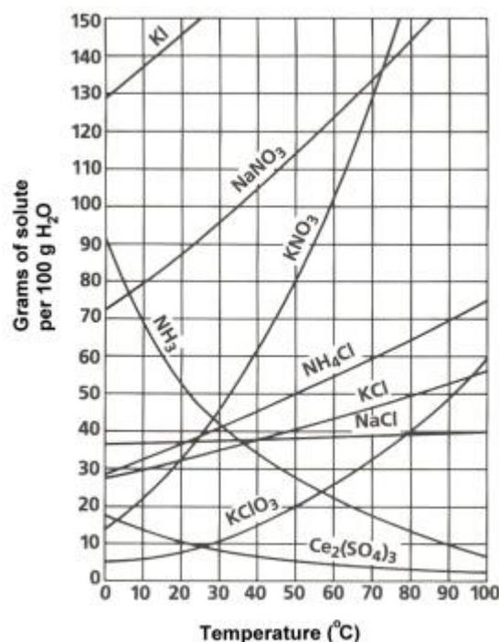
Here's an example of reading the chart. Find the curve for  $\text{KClO}_3$ .
